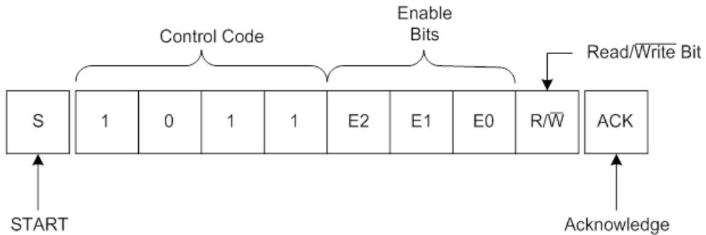
Upon receiving the correct control code, the chip enable bits, and the R/W bit, the device performs an acknowledge by pulling the SDA line low during the 9th clock pulse. As stated above, the device is now set for either a read or a write operation by the R/W bit.
