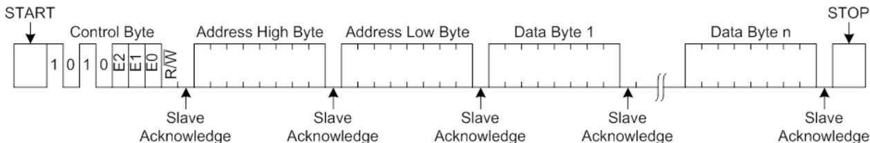
Figure 7-2. Page Write Cycle Timing
